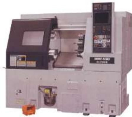
Numerically controlled (NC) machine tools were the first examples of machine tools that used varying degrees of automatic and semi-automatic controls. Nowadays computers are widely used in technology for several applications that include: controlling machines, controlling robots designing articles, producing drawings, simulating, etc.
